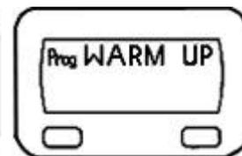
**"COOL DOWN" must be selected in case of air-conditioner** being connected. Only then the activated thermostat-control is able to cool the inside-temperature by switching on the air-conditioner.
