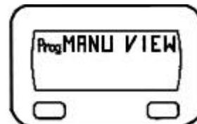
MANU VIEW displays the detected values of one sensor, which later on can be selected by key A.
