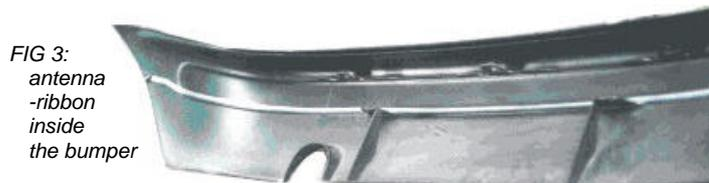
Connect the ribbon to the antenna-flex by the flat-connector. Reinforce fastening of the ribbon, especially at its bends, ends and its connection to the flex (which requires waterproofing, too). It is advisable to cover all the zone of application of the ribbon with plastic protection primer or silicone sealant.
