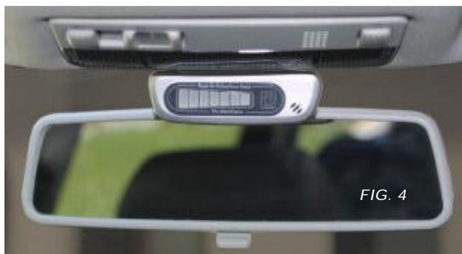
Pass the appr. 4m long 3-wire-cable from the central unit to the display, using opportune passages such as plastic or rubber borders. And connect this cabling to the appr. 1m long cable of the display by using their plugs. (If need be, a prolongation-cable is available optionally.)
